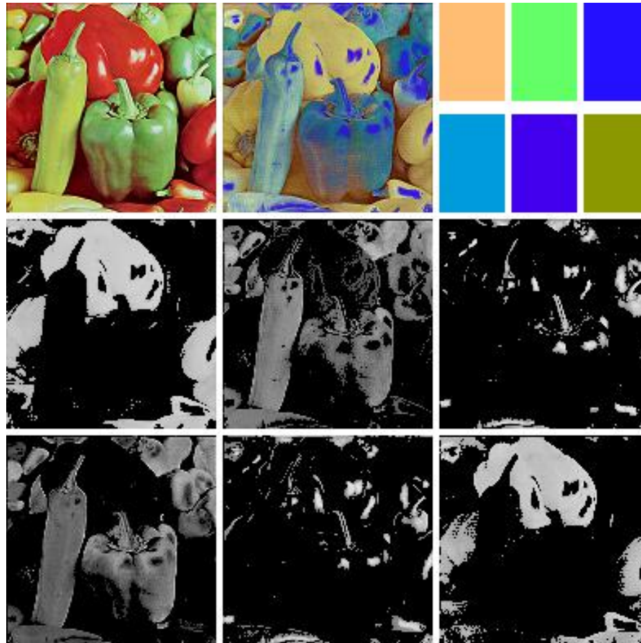
Figure 3. 1st row: RGB color image, transformed HSI color image, saturated colors obtained from the scaled columns of \overline{W} and \overline{M} ; 2nd and 3rd rows: grayscale segmented images derived from \overline{W} and \overline{M} .
