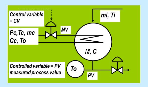
The supervised heat exchanger process scheme
