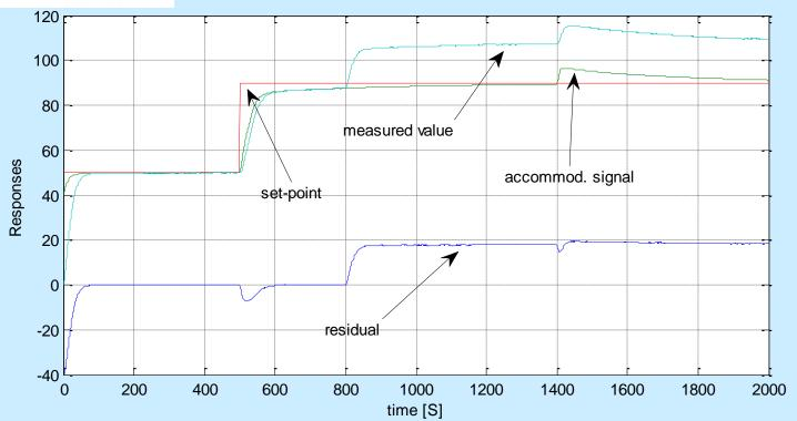
After the fault is detected, the feedback controller tray to avoid the control error but the measured value doesn't reach the set-point value.
