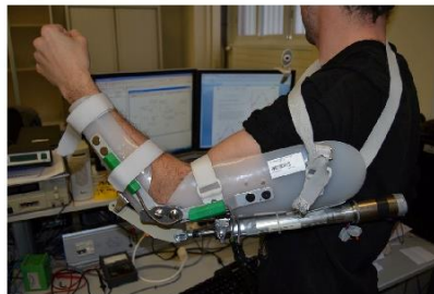
Fig. 1. Custom made arm orthosis.
