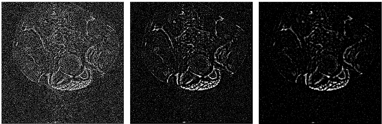
Figure 12. Borders detected in the images filtered with Gaussian Filter method and several neighborhood/radius sizes (threshold 12).
