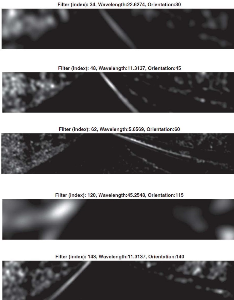
Figure 4.7: Examples of filtered images with Gabor filters of various orientations and scales.
