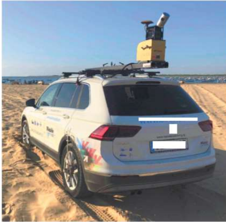
Figure 1.1: The ladybug sensor mounted in a car.
