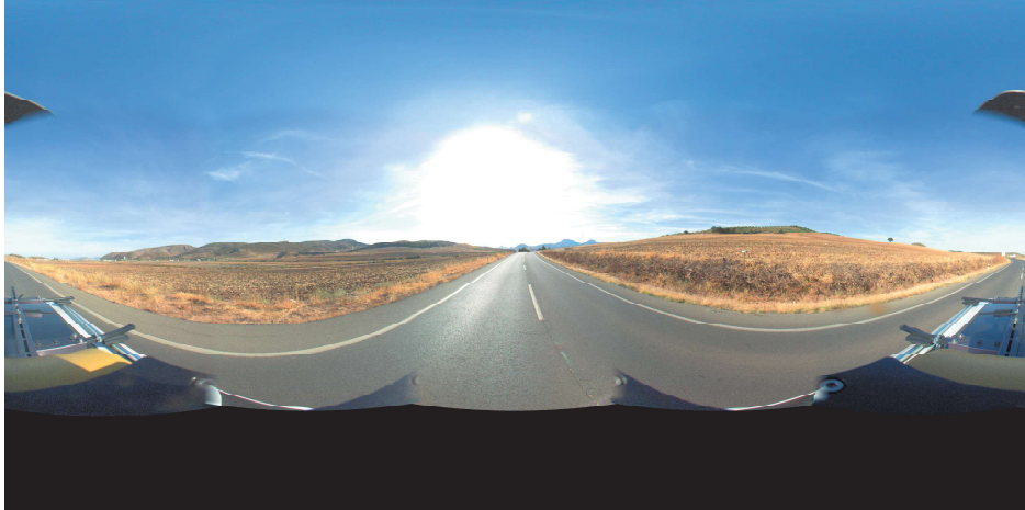
Figure 3.2: An example panorama image obtained from the ladybug sensor after stitching the 6 camera images.
