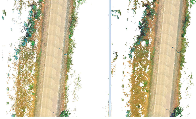
Figure 2.4: Left: RGB point cloud. Right: generated 2D image
