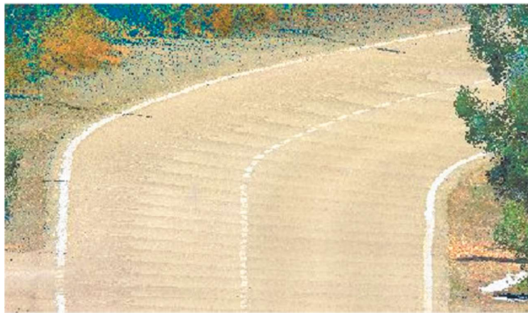
Figure 2.3: RGB image composed by the corresponding RGB pixels to each sample in the LiDAR point cloud.
