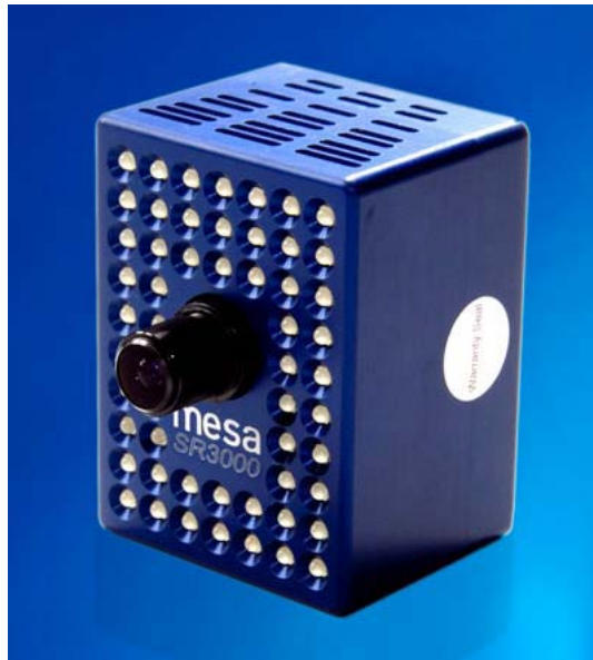
Fig. 1. Swiss Ranger SR-3000 range camera
