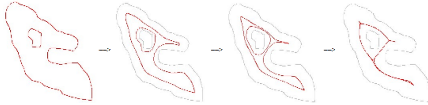
Figure 3.8: Thinning . Thinning iteration example. Red lines correspond to the peeled shape at each step.
