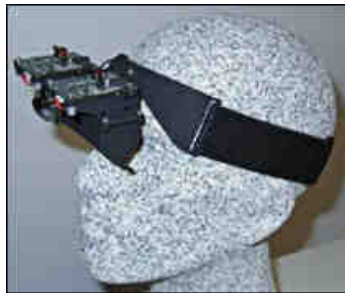
Fig. 12. See-through Head Mounted Display with digital camera attached (Trivisio Prototyping GmbH).
