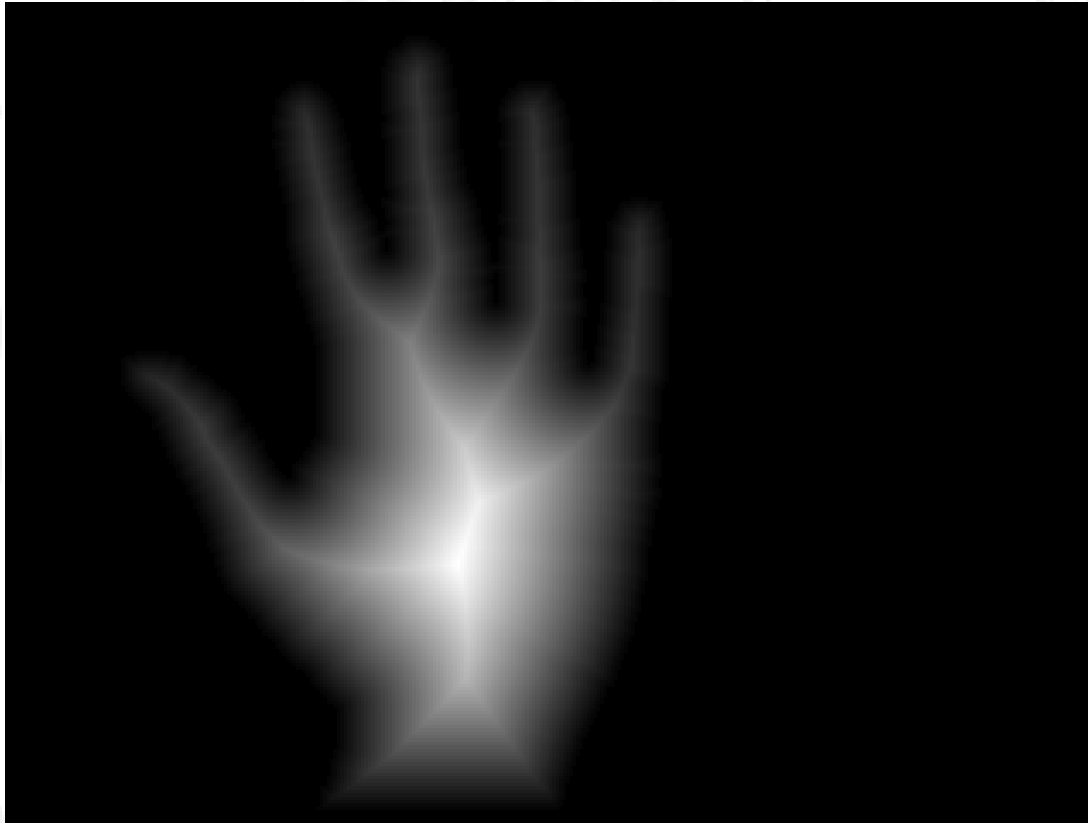
Fig. 3.2: Hand shape Distance Transform Function.
