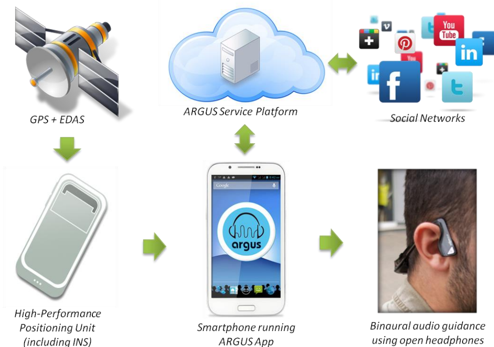
Figure 4.10. Architecture of the ARGUS autonomous navigation system for blind people [Carrasco 2014a].
