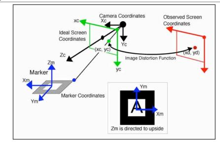
Figure 10.9: AR Toolkit concept and some of the characteristics modeled in the Device Layer.
