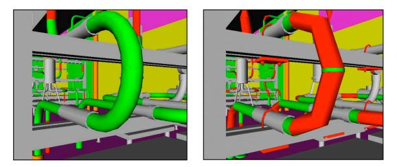
Figure 4.4: User Semantics used for visualization: Different valid graphical representations for a Pipe element
