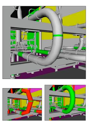
Figure 9.4: Elbow complete (above), reducing the number of segments (lower – left) and dropping holding clamps (lower-right)
