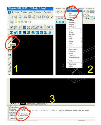
Figure 8.1: Accessing a simple CAD command, 1. Through a button, 2. Drop Down menu, 3. Command line
