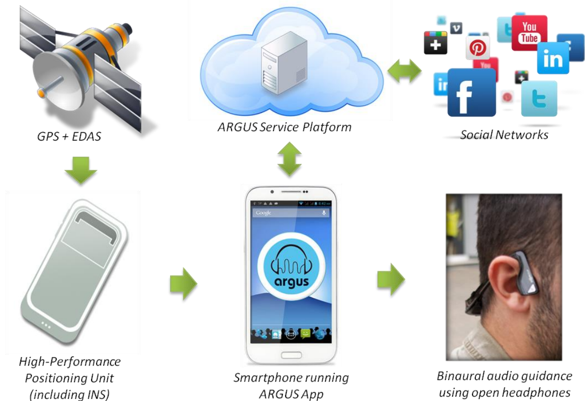
Figure 4.9. Architecture of the ARGUS autonomous navigation system for blind people [Carrasco 2014a].
