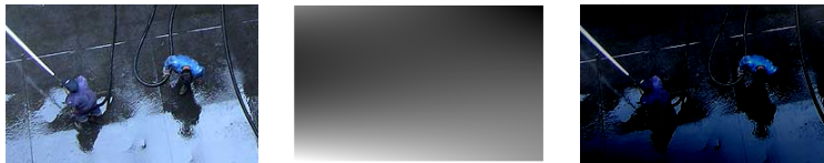
Figure 3.7: Detail from figure 4 images. From left to right: original image, estimated specular bias, corrected image obtained removing the specular bias.
