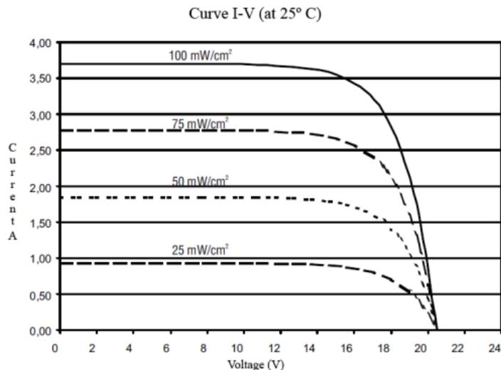
Figure: I-V curve of the Atersa A-55 photovoltaic module
