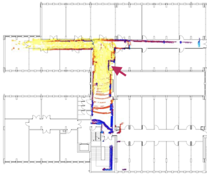
Figure 5.1.5: Projection of the NDT registered point cloud of in-house dataset #1 on the plan of stage 3 of the building.
